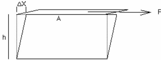
Here  $F$  is a force that I'm applying to slide the top of this block while the bottom of the block is fixed in place.  $A$  is the area over which I apply the force,  $h$  is the height of the material, and  $\Delta x$  is the amount that I manage to slide the top away from the bottom. The "shear strain" is defined as  $\Delta x/h$ , so you can guess what the definition of  $\mu$  is going to look like:
