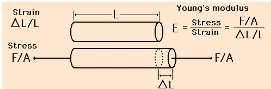
Like the bulk modulus,  $Y$  is defined in terms of stress/strain. Higher  $Y \rightarrow$  harder to stretch. The units are again pressure units (e.g. pascals or  $N/m^2$ ). Numerically, the definition of  $Y$  is:
